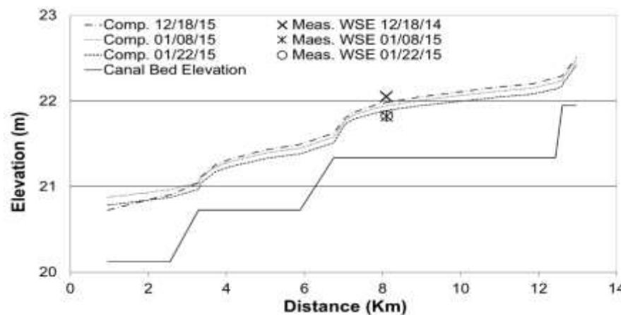
Fig. 9. Computed water surface profiles comparison with measurements
