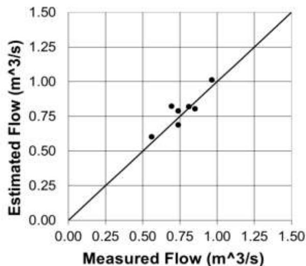
Fig. 2. Comparison of canal flows between estimation and measurement
